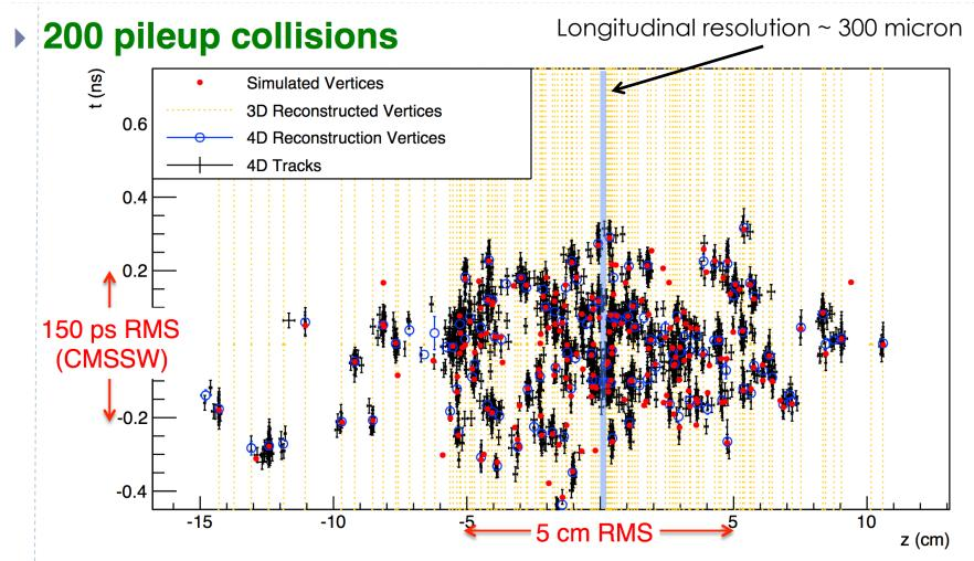
HL-LHC baseline (as of ECFA):  $t_{RMS} = 180 \text{ ps}, z_{RMS} = 4.8 \text{ cm}$
