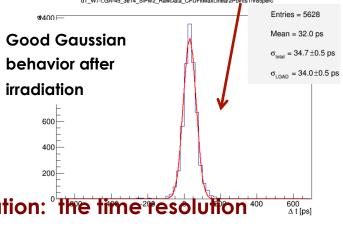
No difference in behavior before and after irradiation: <sup>1</sup>The time<sup>2</sup>resolution<sup>40</sup> <sup>40</sup> scales with gain. → Keep the gain high
