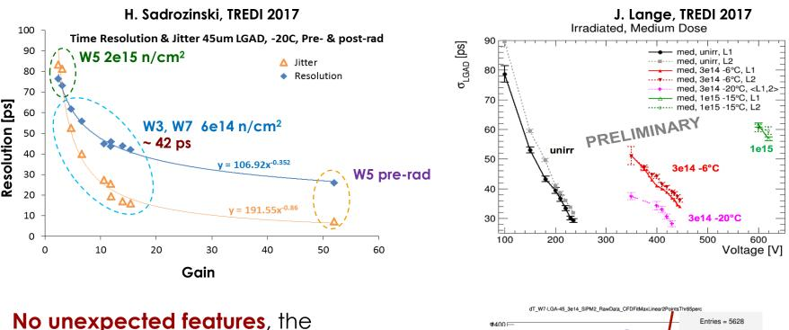
signals are still large and the leakage current does not prevent to reach good time resolution.
