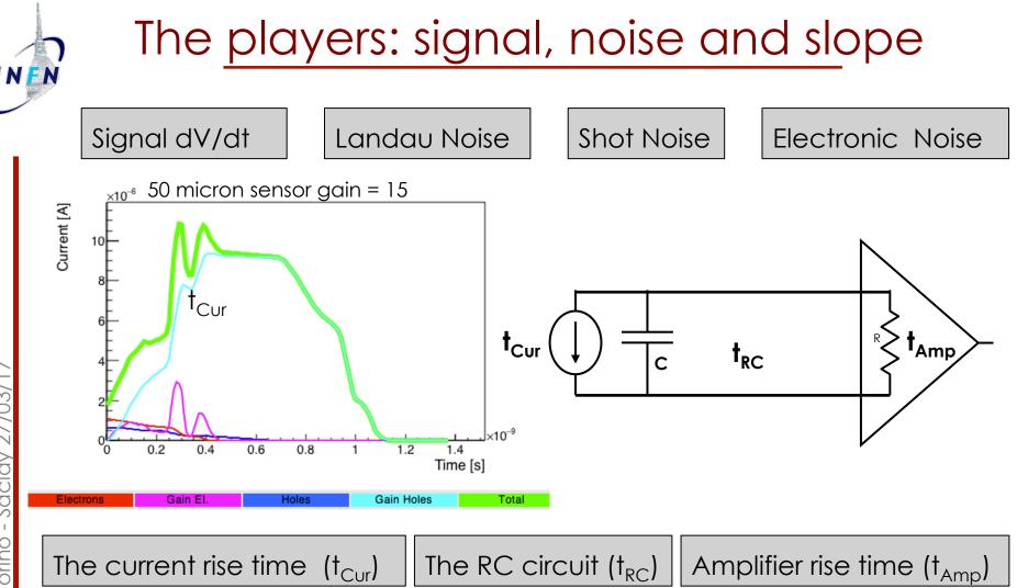
There are 3 quantities determining the output rise time after the amplifier:
