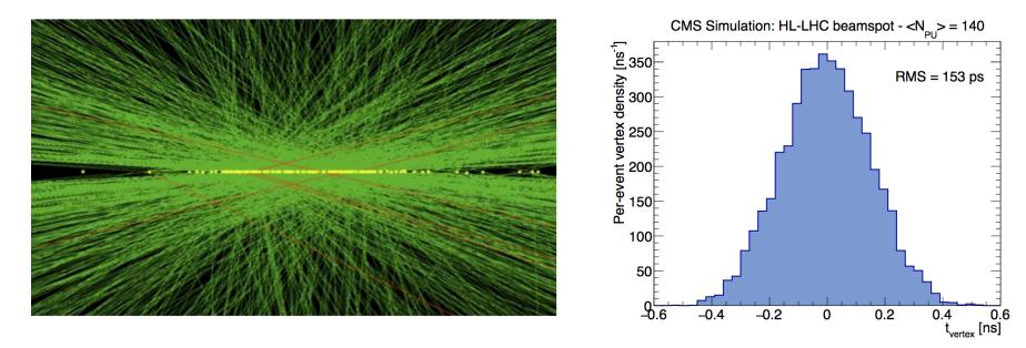
There are between 15-20% of tracking vertexes (longitudinal resolution ~ 200 micron) that are actually composed by 2 or more interactions
