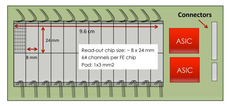
**From physics**: what is the granularity? 1x1 mm2, 1x2 mm2, 1x3 mm2. Shall we use hexagon to minimize the perimeter?
