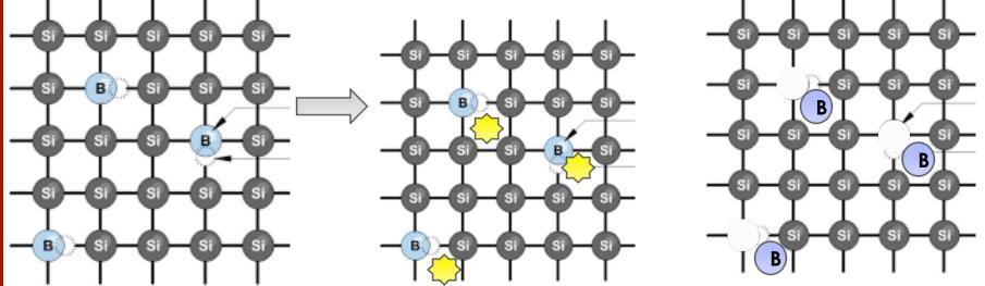
The boron doping is still there, only it has been moves into a different position and it does not contribute to the doping profile, it is inactive
