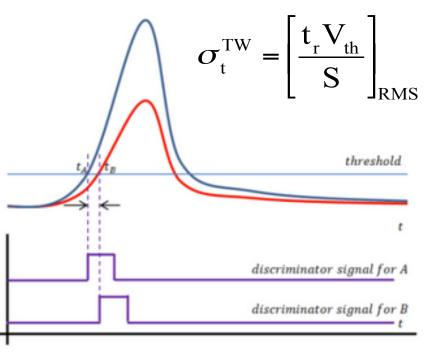
Jitter: the noise is summed to the signal, causing amplitude variations
