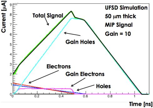
Electrons multiply and produce additional electrons and holes.
