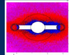
MARS energy deposition map for 1.5 TeV collider dipole
