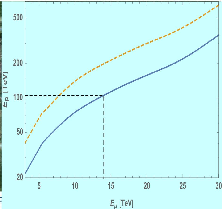
**Figure 1:** The energy at which the proton collider cross-section equals that of a muon collider. The dashed line assumes comparable Feynman amplitudes for the muon and the proton production processes. A factor of ten enhancement of the proton production amplitude squared, possibly due to QCD production, is considered in the continuous line.
