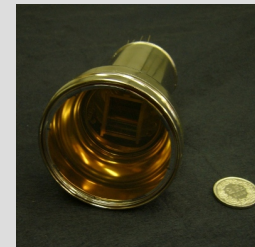
Low Radioactivity Photon Detectors (3", Total ~250)
