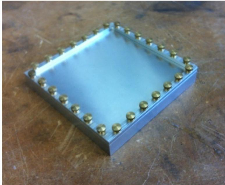
Vibrating clamped plate
