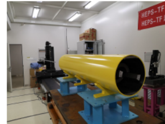
1m long test booster dipole magnet without iron core completed in Oct. 2019, under field measurement
