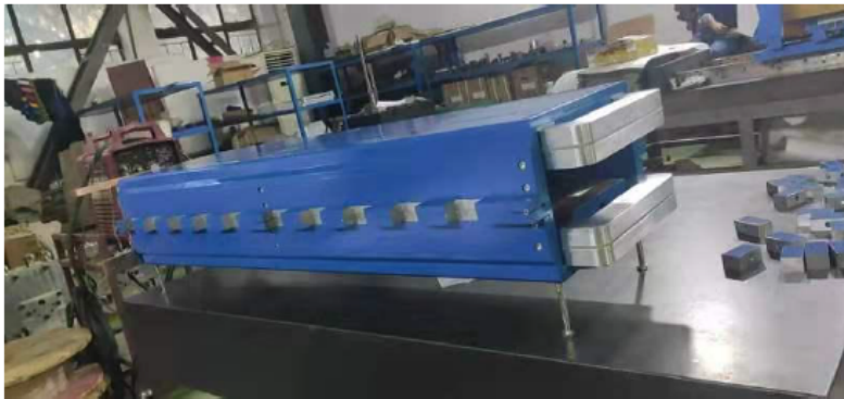
1m long test booster dipole magnet with iron core, completed in Nov. 2019
