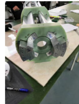
1m long test booster dipole magnet without iron core completed in Oct. 2019, under field measurement
