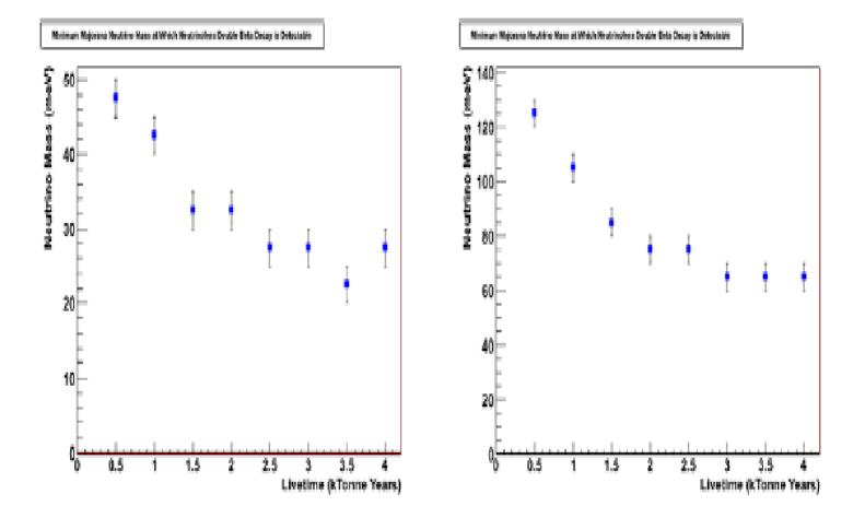
Fig. 4. Sensitivity to neutrino mass reached versus livetime for enriched Nd (left) and for natural Nd (right) in SNO+ from fitting the endpoint spectral shape
