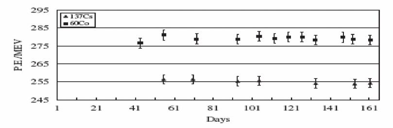
Fig. 6. Long-term stability monitoring of Gd-loaded scintillator by the energy response of the prototype detector to radioactive sources (located at the center of the detector).
