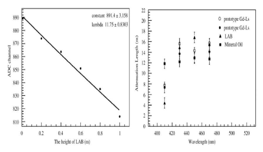
Fig. 4. Left: an example of the attenuation length measurement using the 1-m tube system. The transmissions of different path lengths (Gauss fitting) are fitted to an exponential curve. *Right*: black dots and cycles are attenuation lengths of the 800 L LAB-based Gd-LS used in the prototype experiment. Triangles are that for pure LAB and squares are that for mineral oil.
