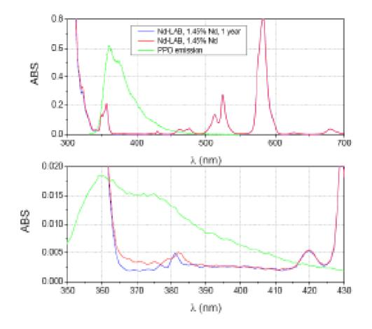
Fig. 1. The absorption spectrum of Nd-LAB scintillator, comparing original data to data taken one year later. The emission spectrum from PPO is also shown.
