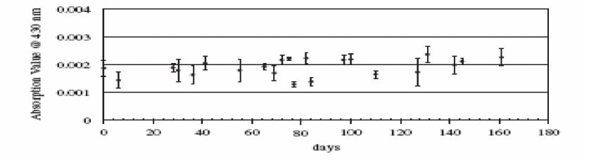
Fig. 5. Absorption of Gd-loaded liquid scintillator at 430 nm as a function of time.
