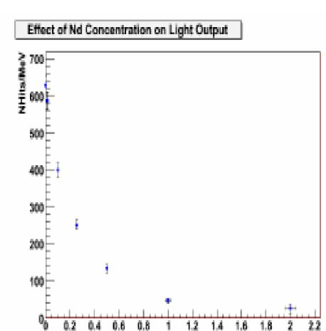
Fig. 2. The effect of Nd concentration on light output. The light output was calculated using a complete scintillation optical model accounting for the propagation of light and using the SNO+ detector geometry and PMT characteristics.
