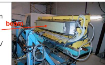
Channel intercalibration with cosmic muons (only Barrel SMs)
