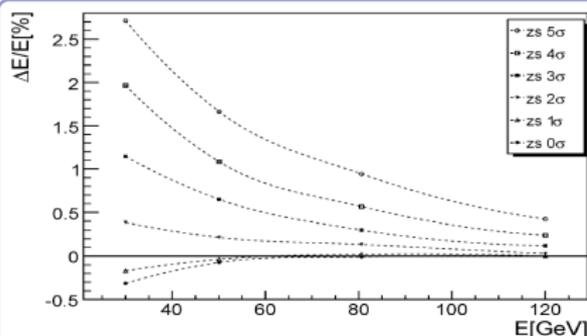
A static zero suppression would introduce a bias on the energy reconstruction.
