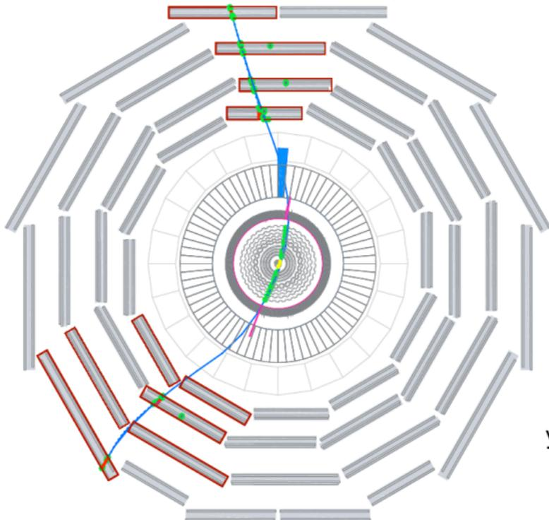
Measurement of the muon **stopping power** in lead tungstate crystals
