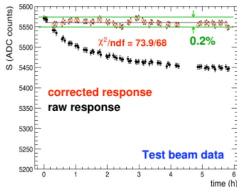
0.2% is the required precision for the target resolution of 0.5% at high energies
