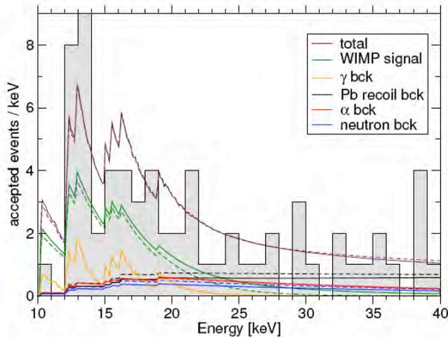
Detailed fit of recoil energy and scintillation distributions + multiplicity (neutrons)
