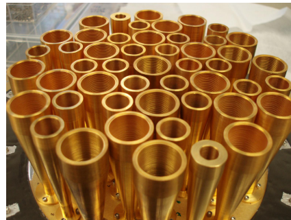
BICEP1: Feedhorns and NTD readout 150 and 100 GHz
