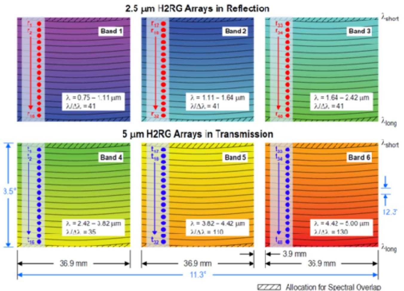
Spectra obtained by stepping source over the FOV in multiple images: no moving parts
