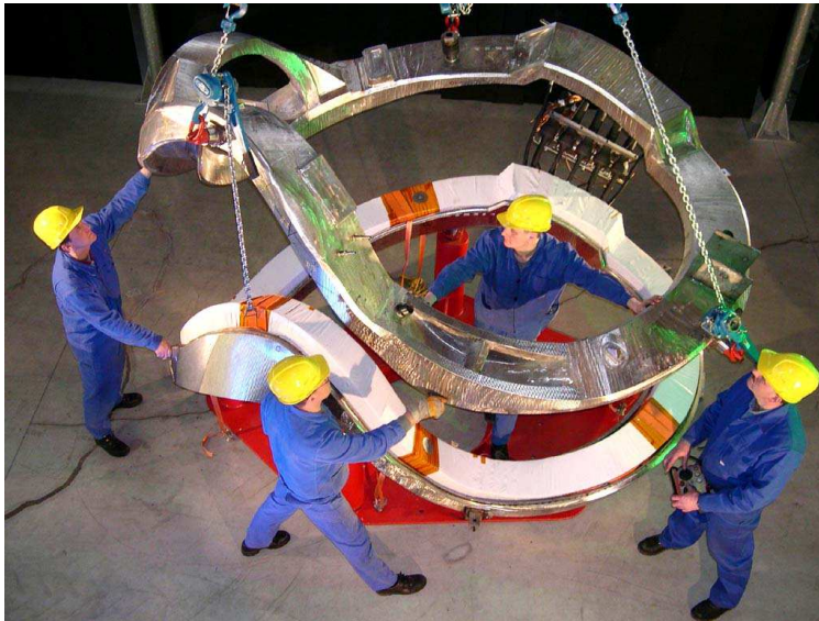
Insertion of Winding in Half Casings
