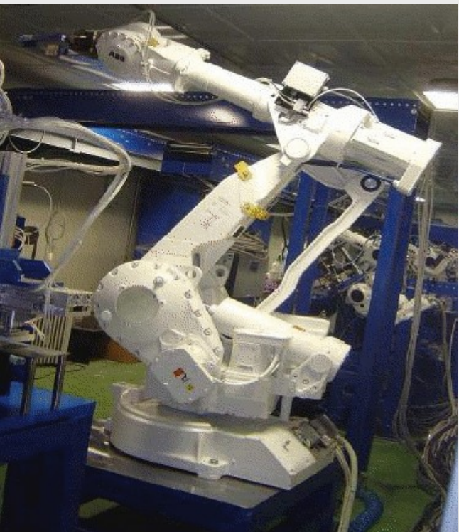
Anthropomorphic robot for brick wrapping
