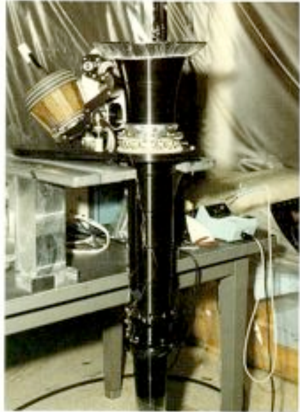
Horn antenna with movable calibrator. Protective plastic covers will be removed.
