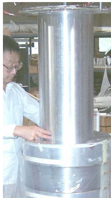
Insertion of the sextupole assembly into the bore of the solenoid bobbin
