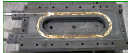
Sub-scale W&R Bi-2212 racetracks with Showa and OST
