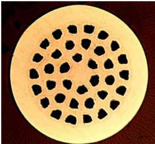
0.87 mm \phi 36-filament wire
