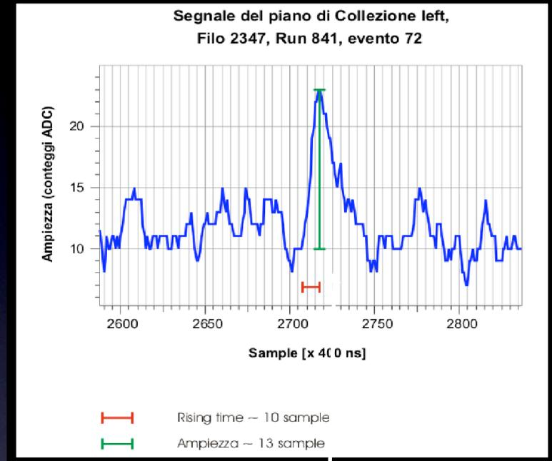
Shapes from  $\text{Fe}^{55}$  radioactive source (5.8 keV, event rate about 1kHz) of the signals from double-stage LEM system have a very clean S/N ratio.
