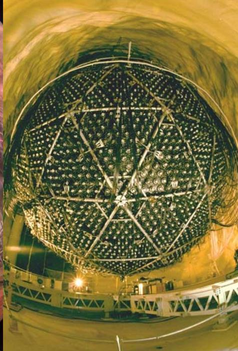
**One million pieces transported down in the 10 foot square mine cage and re-assembled under ultra-clean conditions.**
