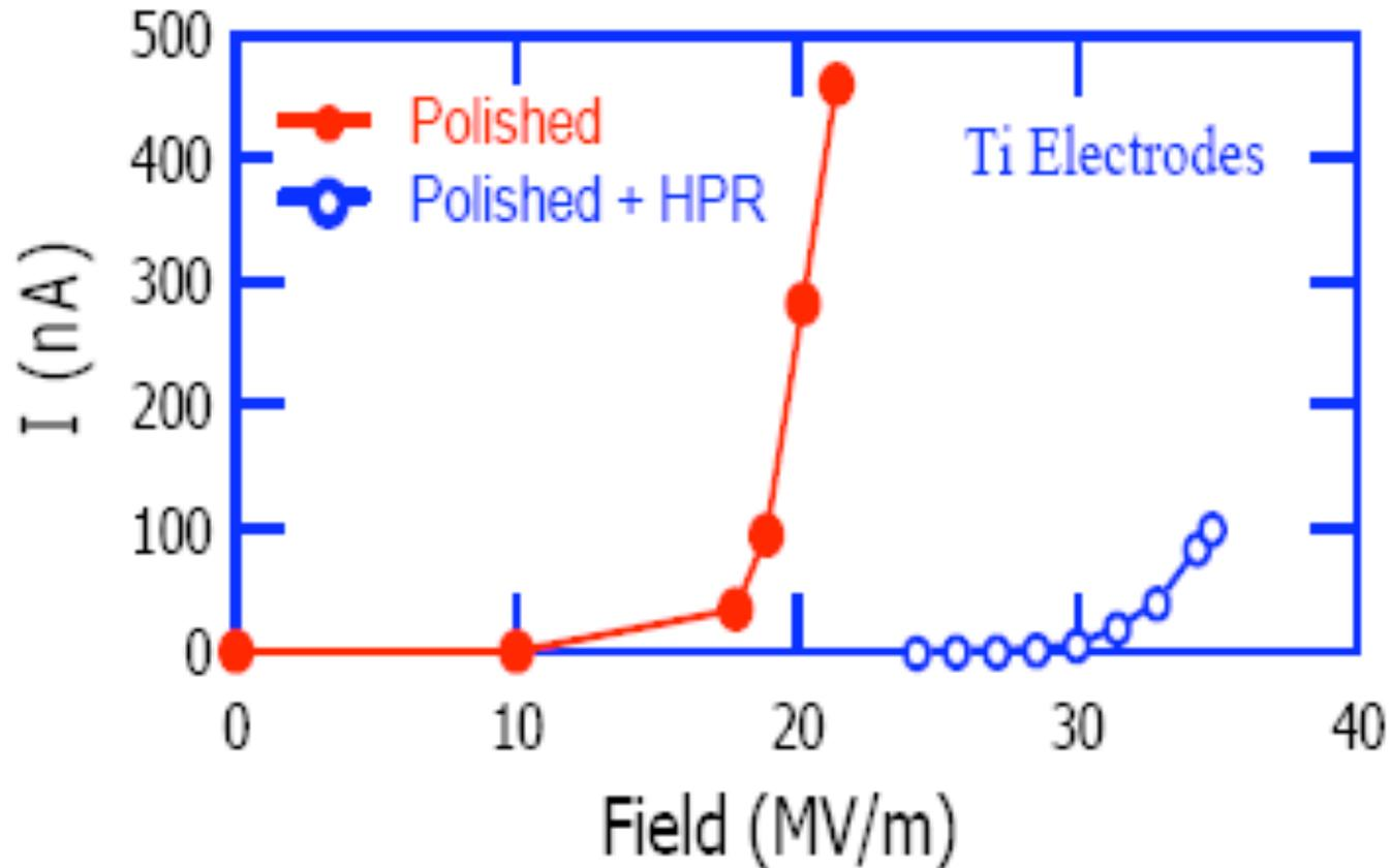
The field emission with and without high pressure water rinsing (F
