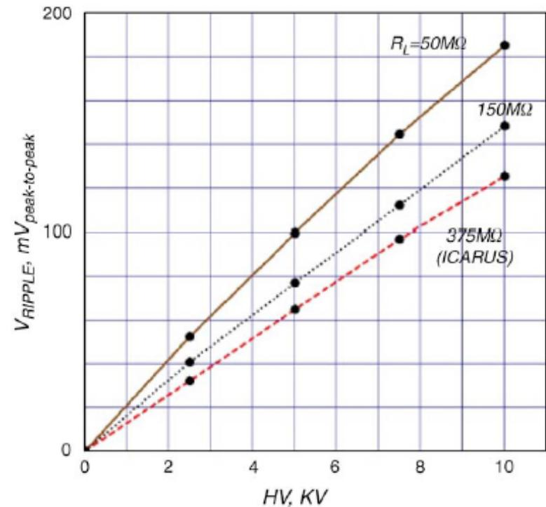
Fig. 41. Dependence of the voltage ripple (peak-to-peak) on the HV for different load resistors. (a) Solid line:  $R_L = 50 \text{ M}\Omega$ ; (b) dotted line:  $R_L = 150 \text{ M}\Omega$ ; (c) dashed line:  $R_L = 375 \text{ M}\Omega$  (T600 working conditions).
