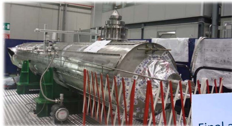
Cryogenic pumping section
