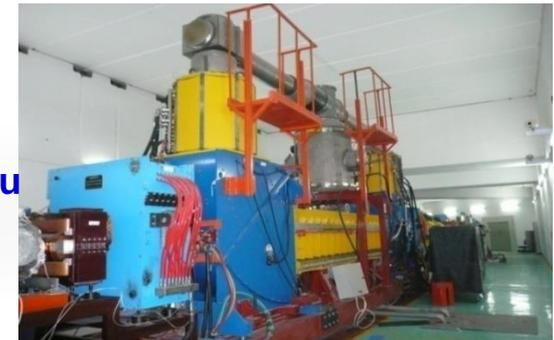
The hollow e-beam can be obtained in both of two e-coolers to partially solve the problem due to the space charge effect and reduce the effect of recombination between the ions and the e-beam. The intensity gain factor of C beam is more than 300.
