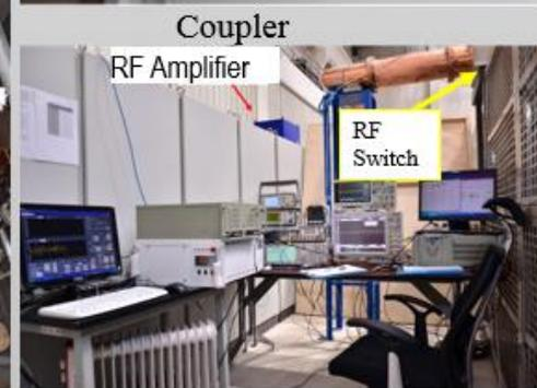
RF components of the RFQ accelerator system
