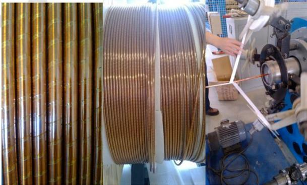
Fabrication of superconducting cable
