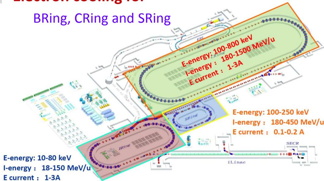
Sketch of the magnetized Electron cooling system for HIAF
