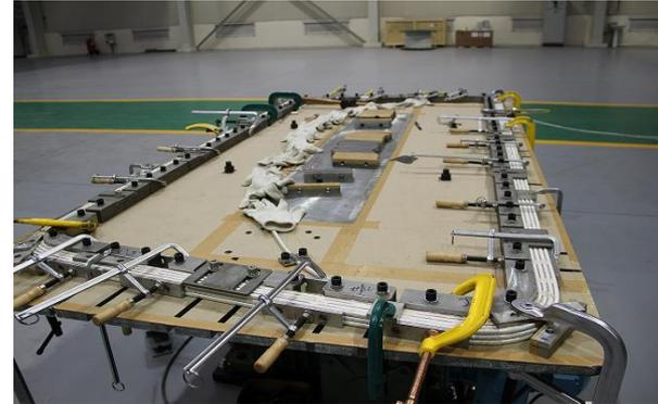
Fabrication of coil case
