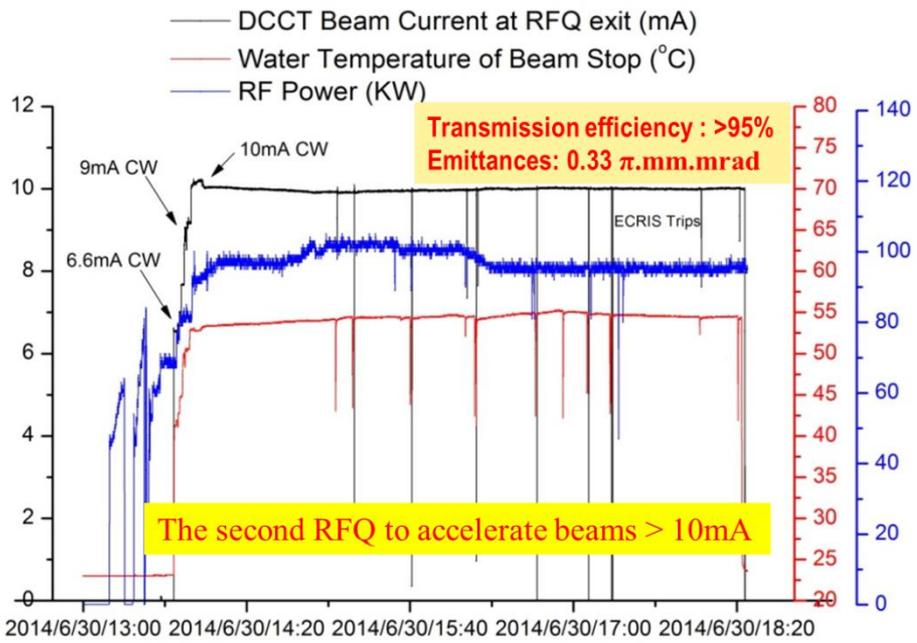
June 30, CW beam @ 10 mA lasted for 4.5 hours
