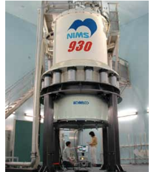
930-MHz NMR magnet (NIMS, 2002) RT bore: 54 mm
