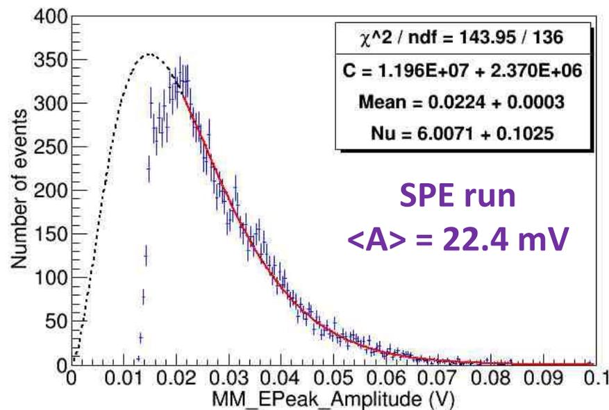
$$\text{Nphe} = 249 \text{ mV} / 22.4 \text{ mV} = 11.1$$
