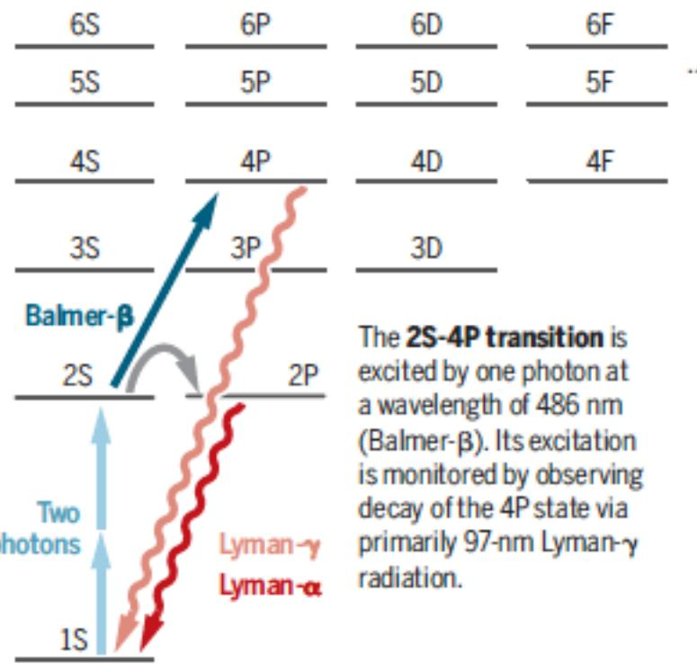
The 2S-4P transition is excited by one photon at a wavelength of 486 nm (Balmer- $\beta$ ). Its excitation is monitored by observing decay of the 4P state via primarily 97-nm Lyman- $\gamma$  radiation.
