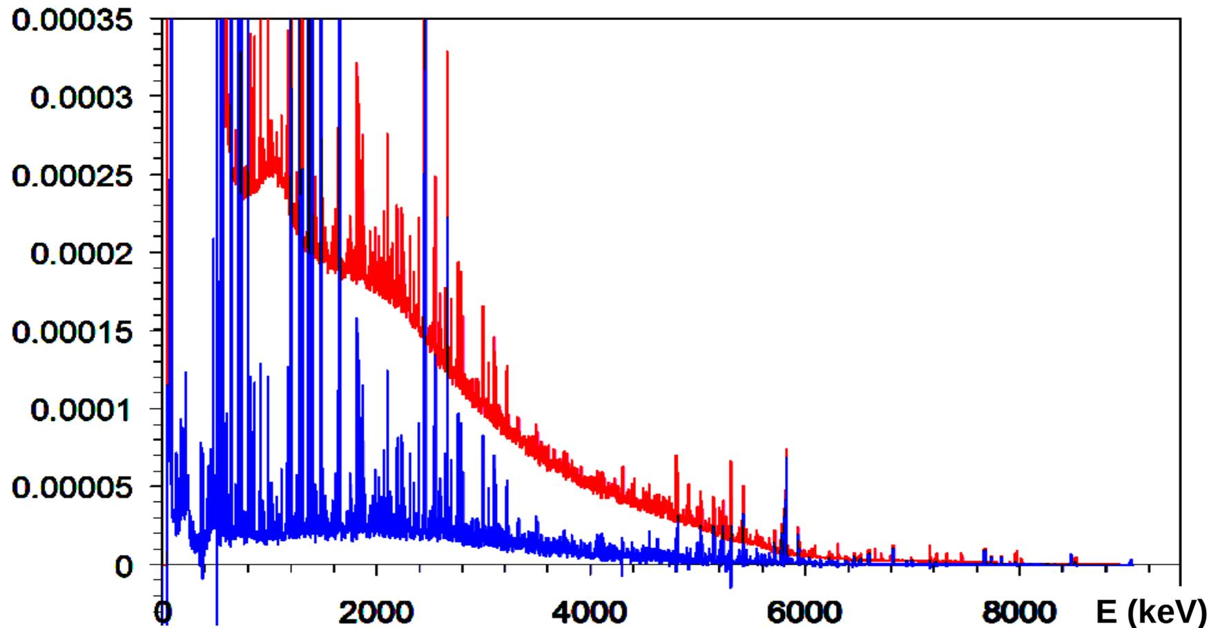
*The deconvoluted, efficiency corrected spectrum shows high level density in quasi-continuous broad distribution peaking at 1 to 3 MeV*
