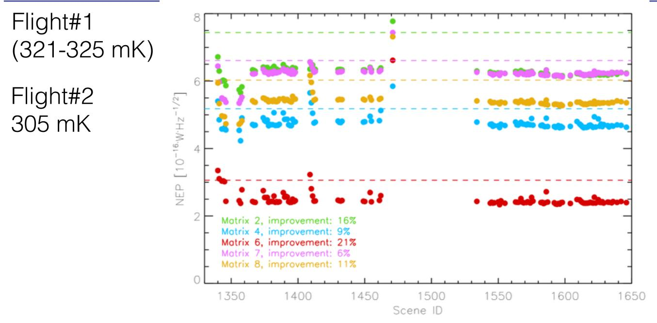
detectors were operated close to 300 mK high frequency noise is 13% better than in flight #1 (equivalent to 26% more integration time)
