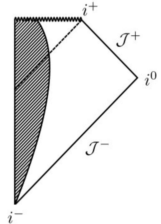
Penrose diagram for a collapsing star
