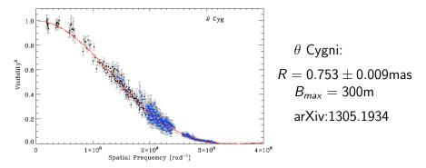
Figure 1. Squared visibility versus spatial frequency for  $\theta$  Cyg for PAVO (blue circles) and MIRC (black diamonds) data. The red lines show the fitted limb-darkened model to the combined data. The solid line is for  $\mu$ =0.47±0.04 (PAVO) while the dashed line is for  $\mu$ =0.21±0.03 (MIRC).
