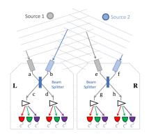
FIG. 3. The two-photon amplitude interferometer. Source 1 sends a photon which arrives as a plane wave at both input detectors "a" and "e". The path length difference leads to a phase offset of  $\delta_1$ , and the photon is in an entangled state (e.g. we recommend Ref. 14)19 for details
