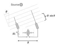
Amplitudes of the signals from two receivers are combined coherently. Interference pattern is correlation vs receiver separation, B
