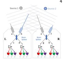
FIG. 3. The two-photon amplitude interferometer. Source 1 sends a photon which arrives as a plane wave at both input detectors "a" and "e". The path length difference leads to a phase offset of  $\delta_1$ , and the photon is in an entangled state (e.g. we recommend Ref. 14/19) for details
