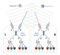
FIG. 3. The two-photon amplitude interferometer. Source 1 sends a photon which arrives as a plane wave at both input detectors "a" and "e". The path length difference leads to a phase offset of  $\delta_1$ , and the photon is in an entangled state (e.g. we recommend Ref. 14) of redetails
